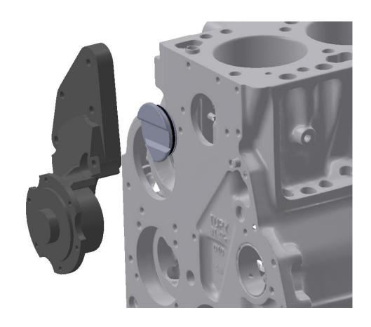
6. Reinstall the factory fan hub and torque the bolts to 18 ftlbs
